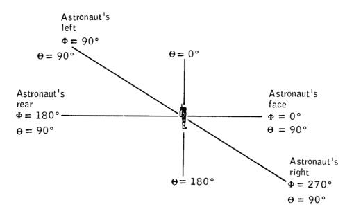
Figure 5. - Pattern coordinate system.
