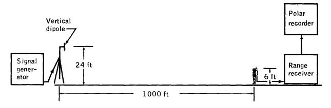
Figure 3. - Antenna pattern setup.
