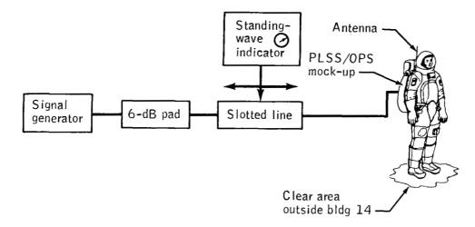
Figure 1. - The VSWR test setup.
